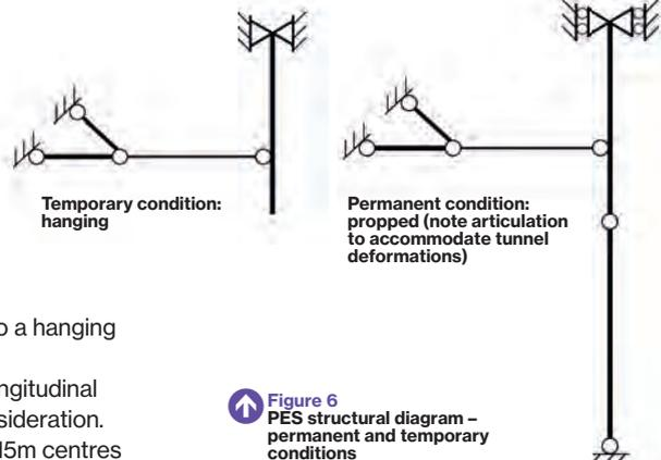
Figure 6 PES structural diagram – permanent and temporary conditions
