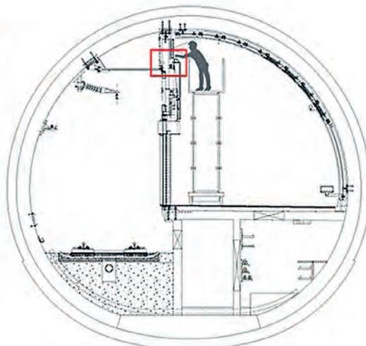
position, without the need for any subsequent operation or curing time. To ensure that delamination in the tunnel lining would not occur, and that the threaded anchors would not loosen or fatigue, Crossrail commissioned testing at Imperial College London. A testing rig was designed to replicate the connection between the PES-frame and sprayed concrete lining and the anchors were subjected to a cyclic load, representative of 10 years in service.
